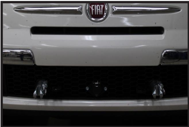
11. Hold the fascia as close to its original position, mark and trim the fascia around the convenience links and attachment tabs. Reinstall the fascia.
