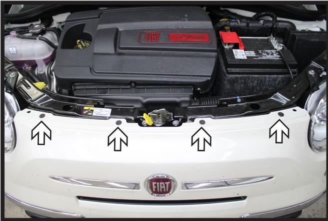
1. Using a T30 Torx, remove the four (4) screws from the top edge of the fascia.
