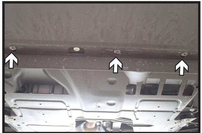
4. Across the center on the underside of the vehicle, use a T30 Torx to remove three (3) screws. **DO NOT** remove the silver screw.
