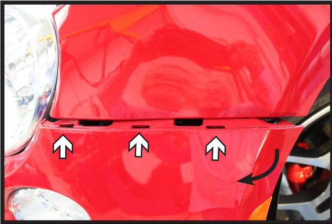
5. Unclip the fascia on the side. Once the fascia has been released, unplug all electrical connections. Next, firmly pull the fascia outward to remove. Set the fascia aside.
