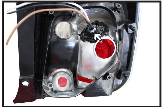
12. Possible location for BX8869 wiring kit: On the side of the tail light, using a T20 Torx remove the four (4) screws. Remove the back piece. Using a 1/2" drill bit, drill a hole in the plastic piece. Put the wires through the hole and silicon around it. Do this on both sides.
