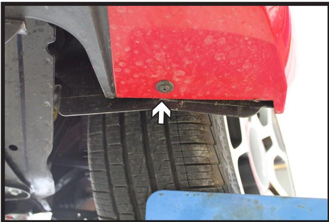
3. Using a Phillips screwdriver, remove one (1) screw from the bottom corner of the fascia. Do this to both sides of the vehicle.
